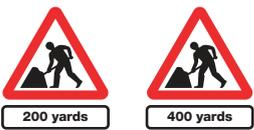
Extra advanced warning signs required for when there is limited visibility on the approach to the works - eg on a bend, brow of a hill, dip in road etc.
