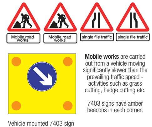
**Mobile works** are carried out from a vehicle moving significantly slower than the prevailing traffic speed - activities such as grass cutting, hedge cutting etc.
